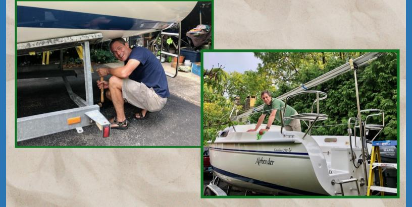
Airbender is a 25' water ballast, swing keel with centerboard; has an 8.5' beam; a hull speed of 6.18 knots and a draft of 5 feet. We sail with a main and a 150% furling Genoa. The keel holds 1,200 pounds of water (that is refilled and drained every time you take the boat in and out of the water, allowing us to power-wash at the Scott Creek boat ramp). By reducing the dry weight of the keel and having a swing keel (as opposed to a fixed keel), the boat is trailerable using our half-ton truck.
